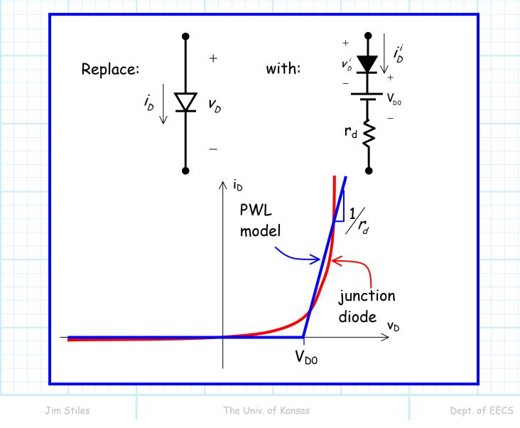
In other words, replace the junction diode with three devices an **ideal diode**, in series with some **voltage source (not** 0.7 V!) and a **resistor**.
